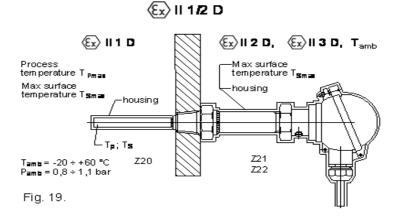
In case of dust explosive atmosphere exists in both side of the process wall and process temperature  $T_p > T_{amb}$ , maximum surface temperature  $T_{Smax}$  occours on the immersion part of the sensor exposed to the process.
