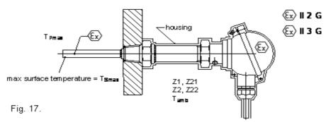
For all sensors except TOPI, TTJI, TTKI, PTTKI, APTOPI, APTTJI, APTTKI, APPTTKI the max process temperature  $T_{pmax}$  must not be higher than the temperature of temperature class for surrounding explosive mixture.
